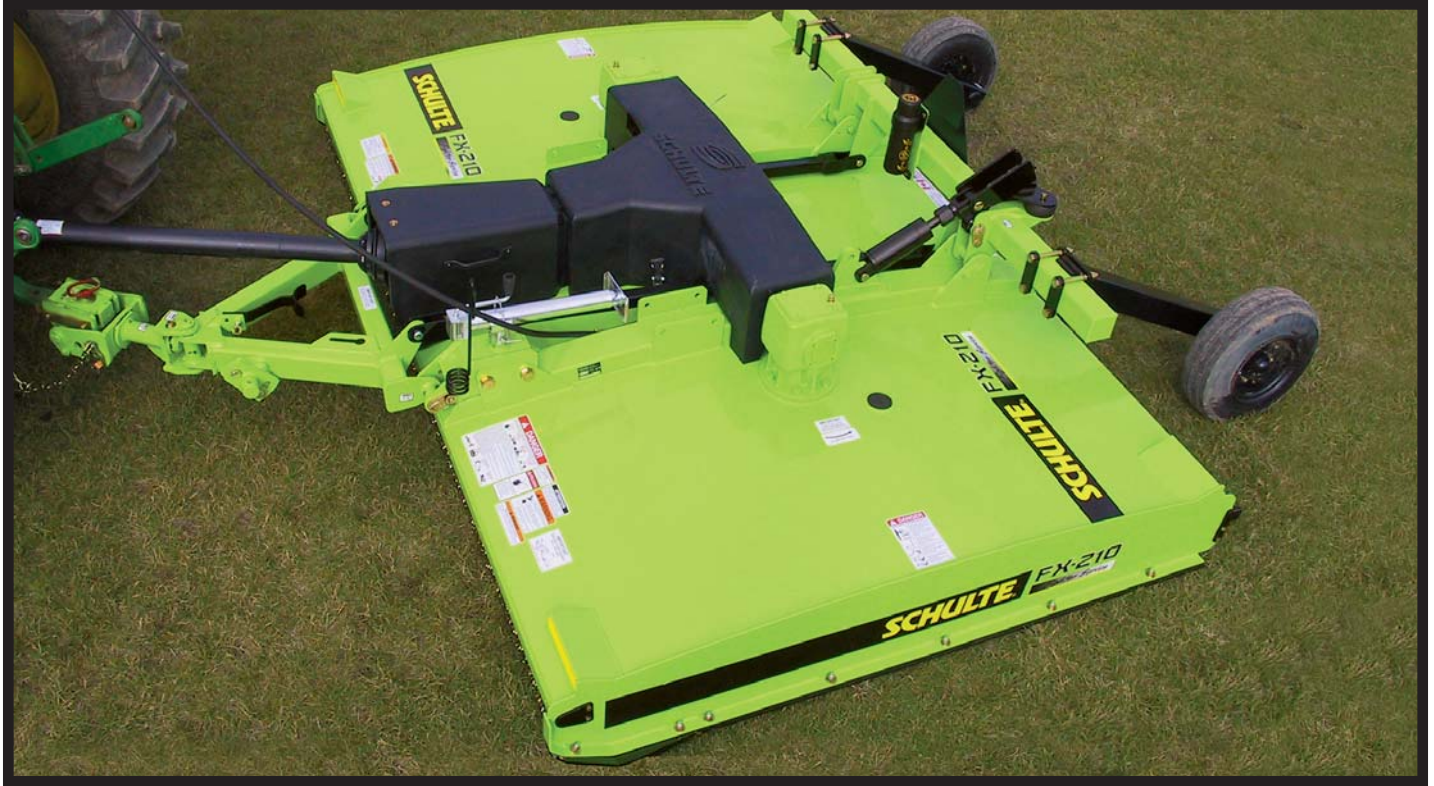
- Trailing unit shown above with non-cv equal angle hitch -
