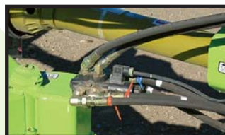
Optional six-port selector valve kit
