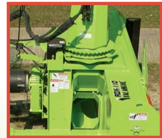
- New gear & motor driven rotator Open right side eject port shown -
