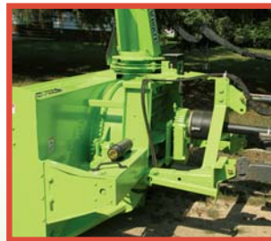
- Heavy duty gearbox & rotating housing mechanism -
