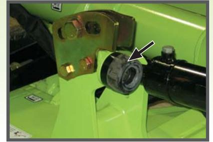
**Wing Lift lock up with rubber stopper**
