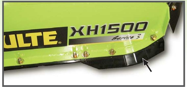
**Side Band Skirt Depth** of 13 3/8" creates maximum flow of cut material
