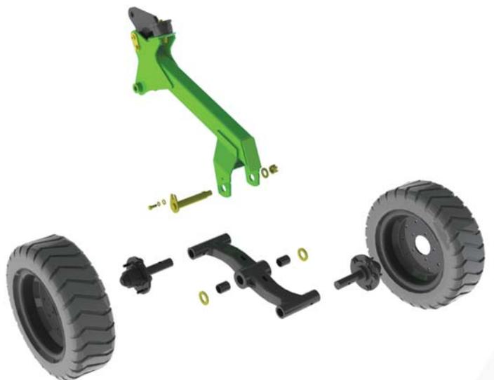
**Swivel Hitch** A swivel hitch allows the cutter to move over rough terrain without the hitch clevis binding up onto the tractor drawbar. The swivel assembly uses a strong 2" main shaft. Should the assembly loosen up over time machine bushings can be added to maintain a snug fit. A spring steel bushing protects the hitch frame from wear.
