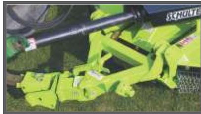
**Wing Suspension** with rubber grommet. Lock head pins with greaseable replaceable spring steel bushings at all major pivot points ensures proper lift height for the life of your Schulze cutter.
