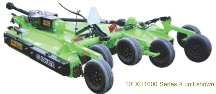
**Drive Line** A four gearbox drive line arrangement with a forward mounted power divider allows the use of individual slip clutches to protect the cutter. The four gearbox drive line allows the wings to operate at angles from 25° down up to transport position.
