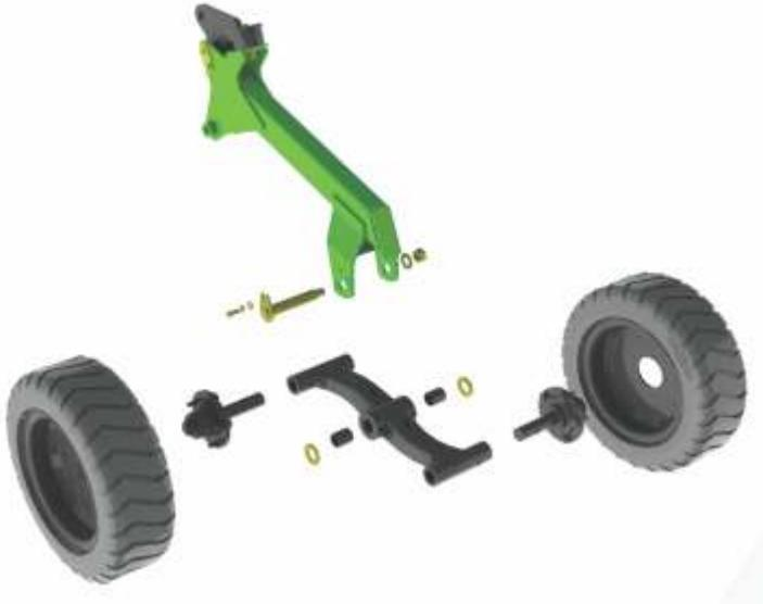
**Swivel Hitch** A swivel hitch allows the cutter to move over rough terrain without the hitch clevis binding up onto the tractor drawbar. The swivel assembly uses a strong 2" main shaft. Should the assembly loosen up over time machine bushings can be added to maintain a snug fit. A spring steel bushing protects the hitch frame from wear. The complete assembly can be changed by removing four bolts.
