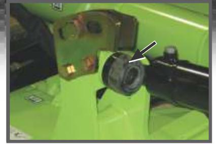
**Wing Lift lock up with rubber stopper**
