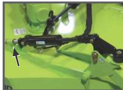
**Leveling** (Industry First) Outer wing wheels include an adjustment screw that can be placed out of level up or down 3". This allows the cut height to be fine tuned across the machine for precision cutting along roadsides.
