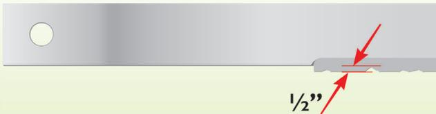
Any nicks or gouges that are over 1/2" deep require the blade to be replaced. Replace blades if normal blade wear exceeds 1/2" from the original size of the blade.
