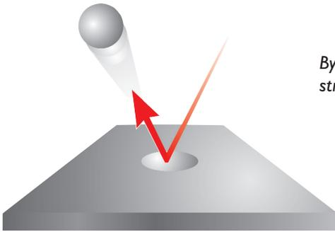
By utilizing a cold working process such as **shot peening**, Schulte is able to provide a compressively stressed blade surface which is highly effective in preventing surface crack formation and propagation.
