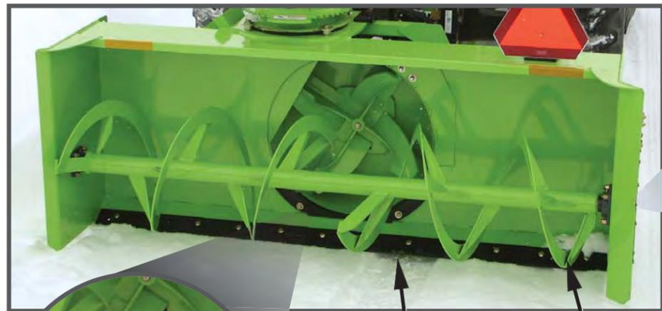
Replaceable cutting blade
