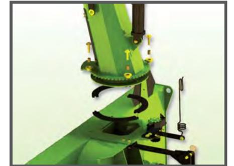
A high molecular UHMW bearing area keeps freeze ups to a minimum in the coldest weather conditions.
