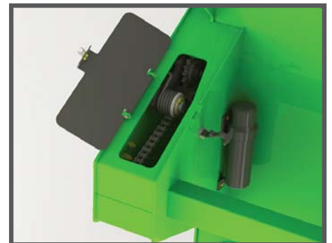
Enclosed chain case with spring tension tightener for idler sprocket maintains constant tension on the auger drive chain & reduces chain wear and possible freeze ups.
