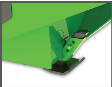
Adjustable replaceable skid shoes are set close to the cutting blade for better ground following. Gauge wheel with tapered roller bearings are optional for use on pavement or cement.
