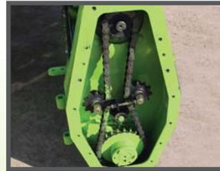
Gearbox features reversible tensioner and heavy 80 chain which decreases downtime. The gear ratio has a larger bottom sprocket that increases the mechanical advantage, giving deeper ground penetration and fewer stall outs. Side plates are adjustable, removable, and reversible for varying ground applications.
