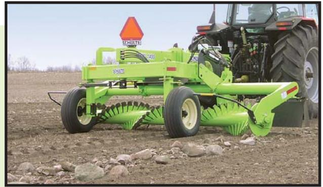
The SRW 1400 Pivoting Rock Windrower employs a side delivery frame arrangement which allows the operator to better control the size of windrows, regardless of rock conditions. The windrower's **patented** floating drum arrangement allows the wheels to be placed closer to the windrower drum, resulting in excellent ground following characteristics.
