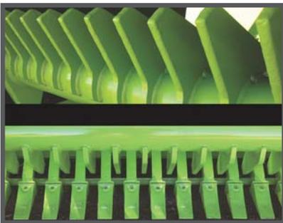
450 BNH steel for heavy duty windrowed picking
