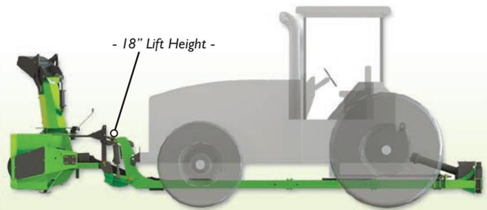
Simple attachment and removal from your tractor. A wide selection of proven tractor mounting brackets are available, for new, or older tractor models. A compact Category 2, 3PT lift mechanism ensures
